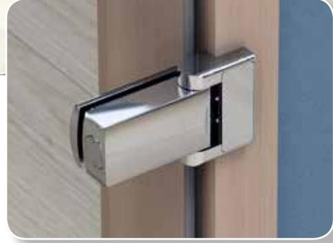
**There are three types dedicated to frames with German standards, for inner tempered glass doors. The hinges are the hydraulic ones of Biloba series and make the adjustment of door closing speed possible. The door movement is completely safe and in case of violent accidental pull, the door does not oppose any resistance. They have undergone many tests, reached over one Million of cycles and certified by TÜV according to DIN 1154:2006.**
